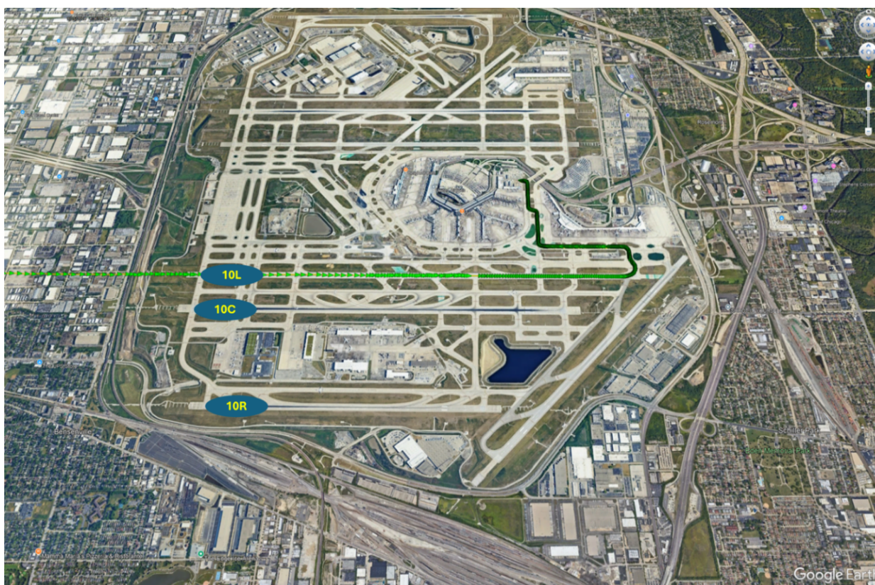
Figure 1. Google Earth screenshot that is overlaid with automatic dependent surveillance-broadcast (ADS-B) ground track showing the incident flight.
