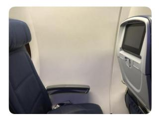
20. One of Delta's competitors, Alaska Airlines, explains on its website: "That's the spot where Boeing places the air conditioning riser ducts from the belly.... The vertical ducts are located behind the passenger compartment sidewall panels and they prevent the installation of a window in one row on the left side. This is standard on all Boeing 737 aircraft, not just ours."
